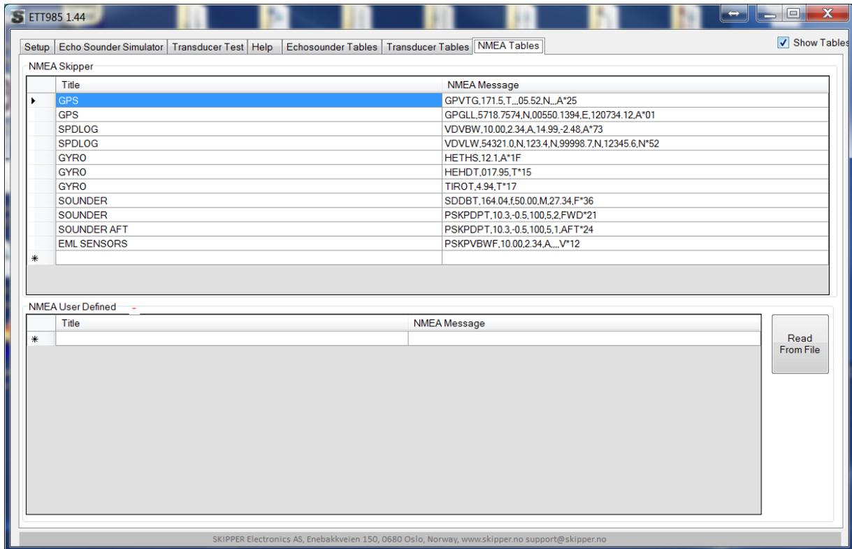
The SKIPPER service software contains tests for echosounders containing test parameters for the return pulse, setup parameters for the sounder under test (for the user to set), limits of the measured pulse, and an expected picture of the screen. Also a comment field that allows an explanation of how to do the test.
